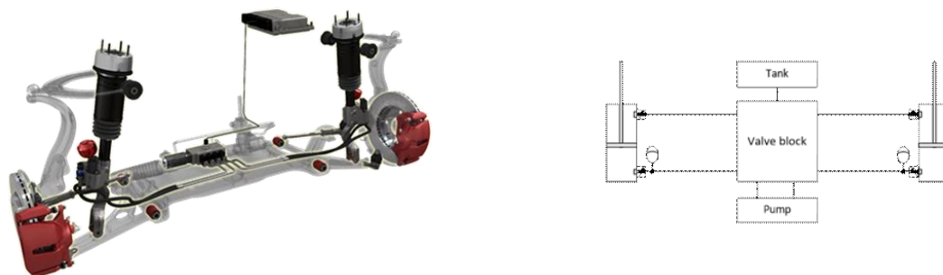
Figure 4: (left) Generic design for the electro-hydraulic suspension, (right) Electro-hydraulic concept
