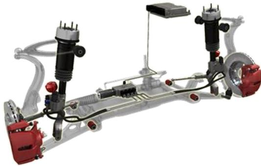
Fig. 5 Active suspension layout.
